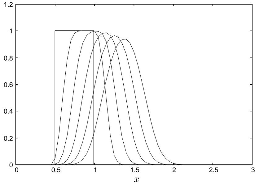
Up-wind scheme (左から右へ  $t = 0, \frac{1}{8}, \frac{2}{8}, \frac{3}{8}, \frac{4}{8}, \frac{5}{8}$  ( $\Delta t = 1/64, \Delta x = 1/20$ ))
