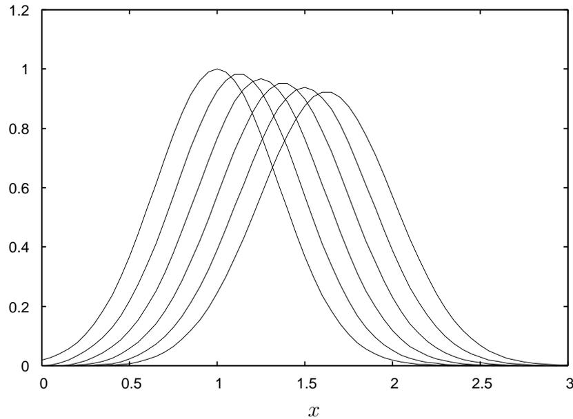
Up-wind scheme (左から右へ  $t = 0, \frac{1}{8}, \frac{2}{8}, \frac{3}{8}, \frac{4}{8}, \frac{5}{8}$  ( $\Delta t = 1/64, \Delta x = 1/20$ ))
